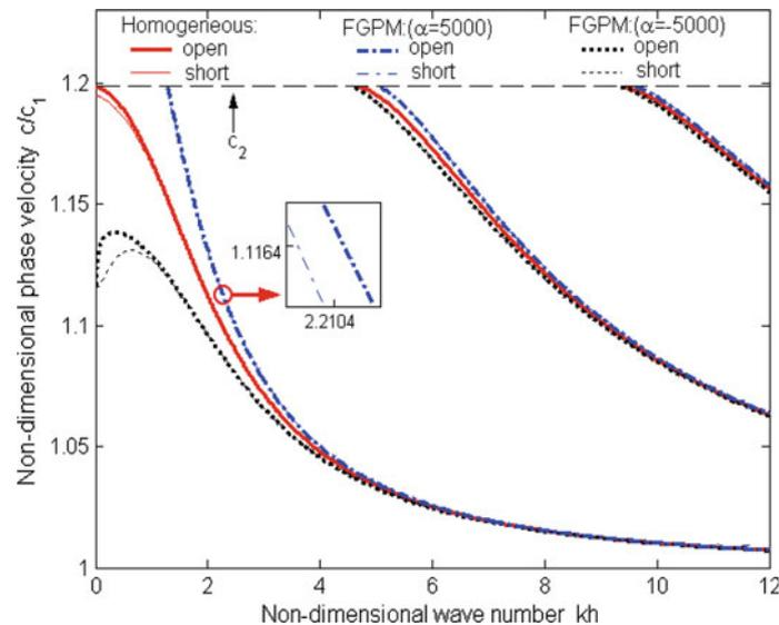
**Fig. 2** Dispersion curves of Pb glass layer/ZnO substrate system with/without material gradient
