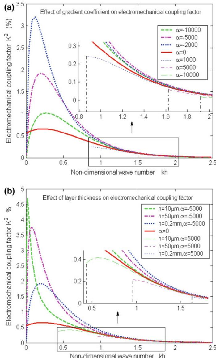
**Fig. 4** Electromechanical coupling factor of the fundamental mode affected by (a) material gradient, (b) covering layer thickness
