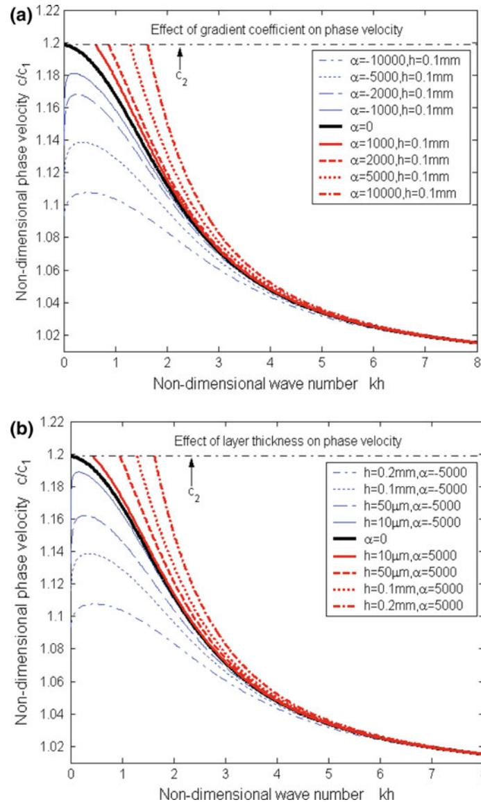
**Fig. 3** Phase velocity of the fundamental mode affected by (a) material gradient, (b) covering layer thickness
