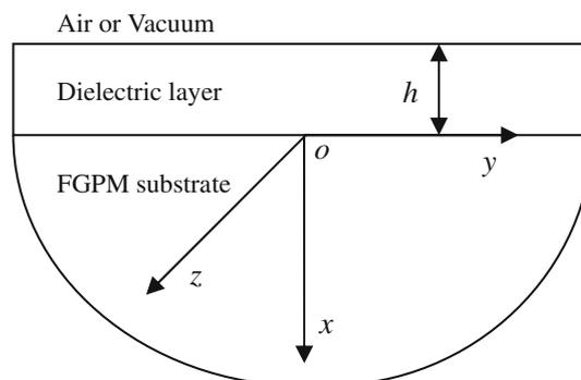
**Fig. 1** A schematic configuration of a layered half-space and coordinate system
