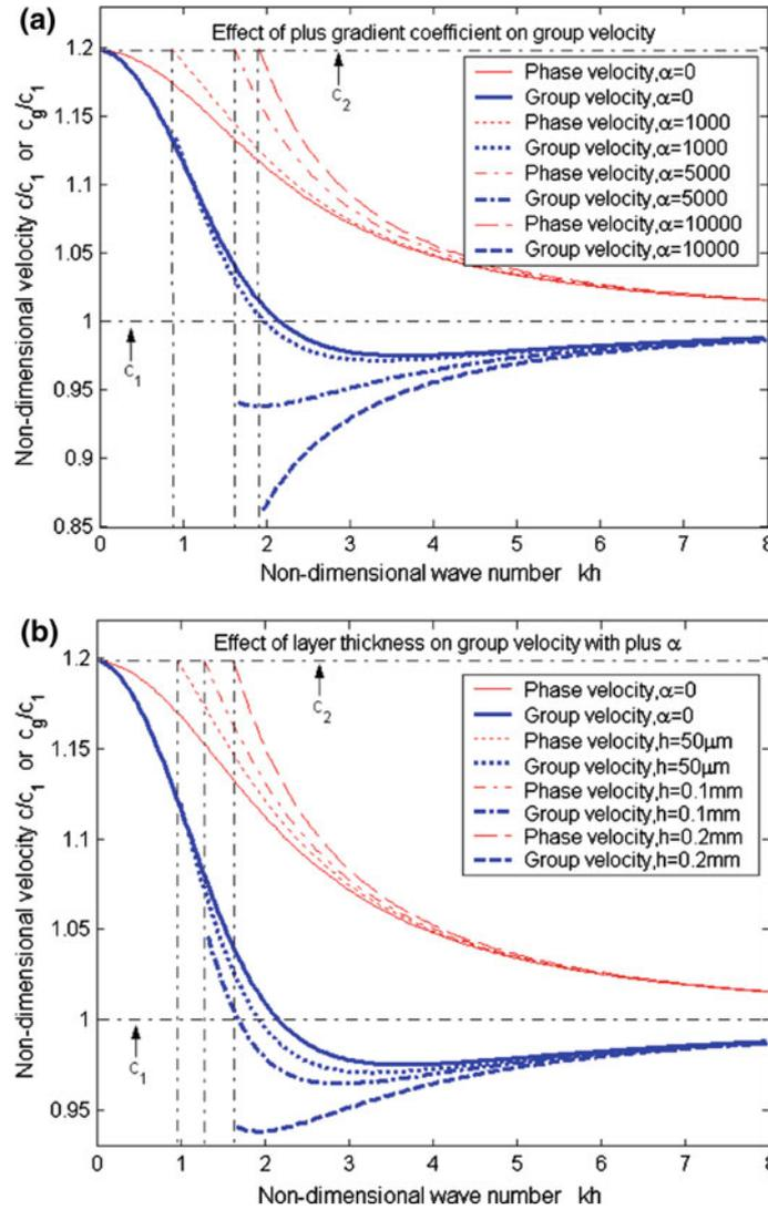
**Fig. 5** Group velocity of the fundamental mode affected by (a) material gradient, (b) covering layer thickness
