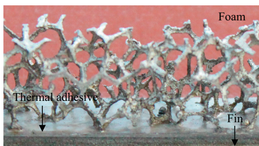
Fig. 2. Enlarged view showing adhesive-bonded interface between metal foam and plate-fin.
