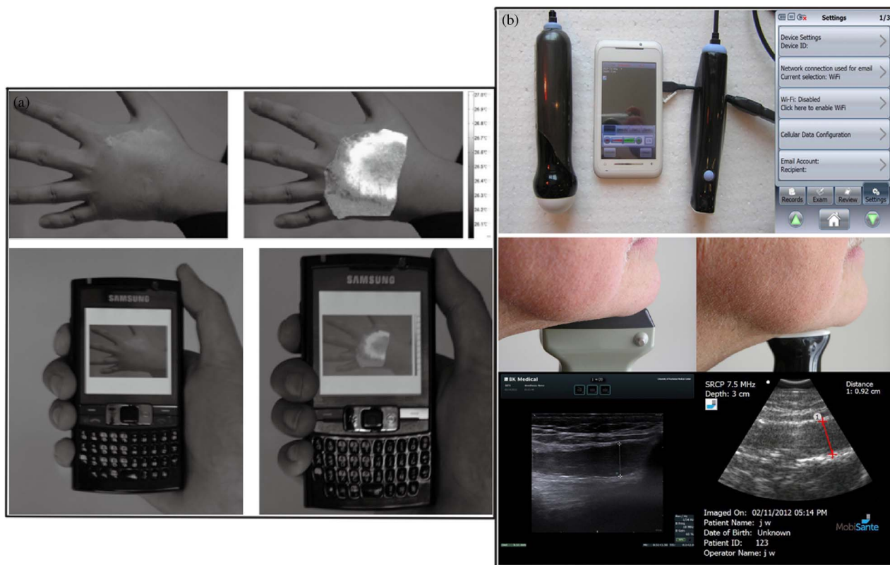
Fig. 2. Examples of in vivo POC diagnostics with extra sensors. (a) Skin temperature detection by mapping skin temperature changes to TLC color changes [42]. (b) POC ultrasound imaging system (MobiSante MobiUS SP1 system) with two mechanical sector USB probes [44].
