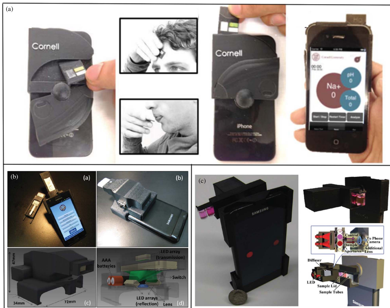
Fig. 4. Direct tube, strip, and specimen inspection for POC diagnostics. (a) Smartphone-based health sweat and saliva biomarker detection device [55]. (b) Different views of the smart RDT reader prototype installed on an Android phone (Samsung Galaxy S II). This device can be repeatedly attached/detached to the cellphone body without the need for fine alignment and modification [56]. (c) A picture of the iTube platform, utilizing colorimetric assays and a smart phone-based digital reader for food allergen testing [58].
